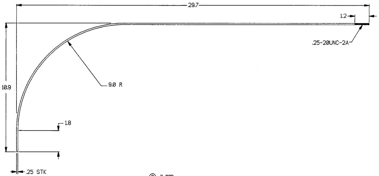
FIG. 8 Shading Disk Support Bar
