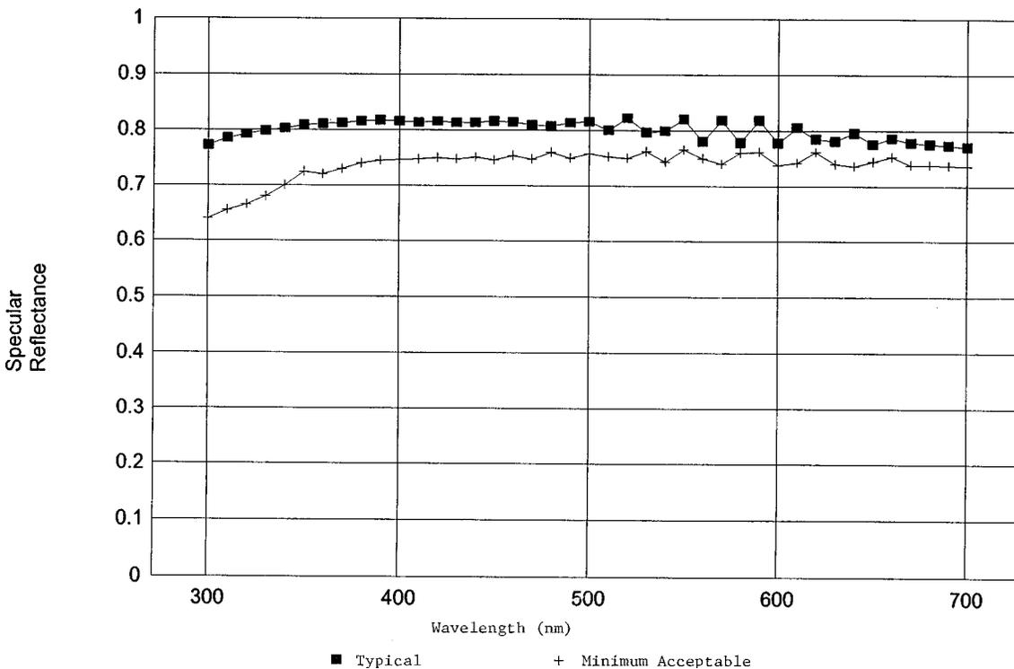
FIG. 4 Specular Reflectance of Mirror Material
